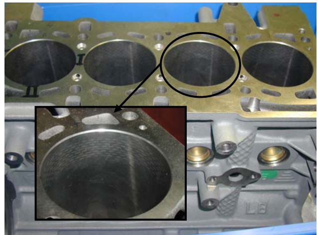
Fig 1 View of typical four cylinder liner engine block of modern car and focus on honed –laser textured surface.
