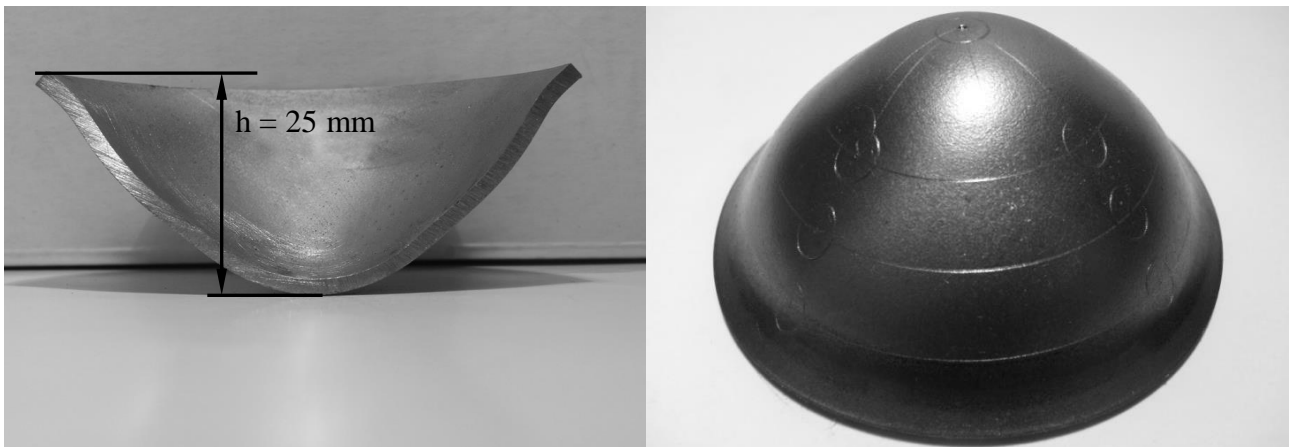
Fig. 17. Drawpiece with a 25 mm height obtained on the spherical punch
