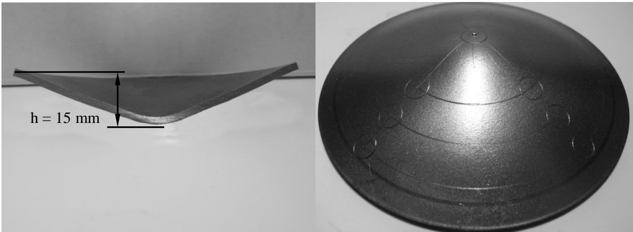
Fig. 16. Drawpiece with a 15 mm height obtained on the spherical punch
