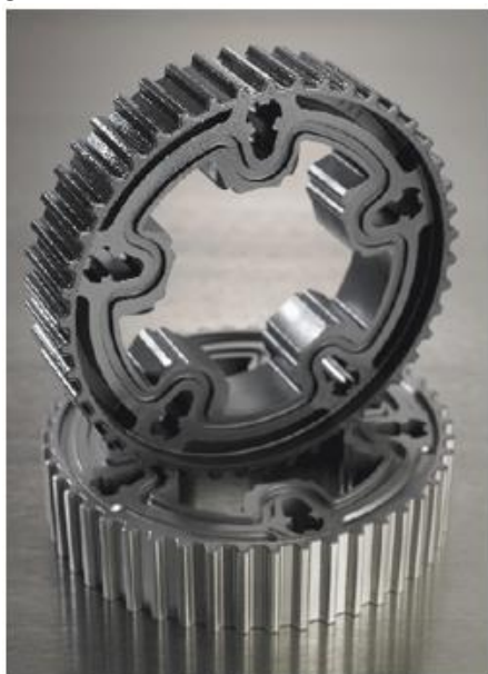
Fig. 2 System stator produced by powder metallurgy for the customer [5, edited and supplemented by author]
