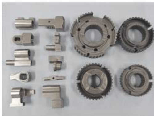
Fig. 1 Example of powder metallurgy components used in automotive sector [1, edited and supplemented by author]
