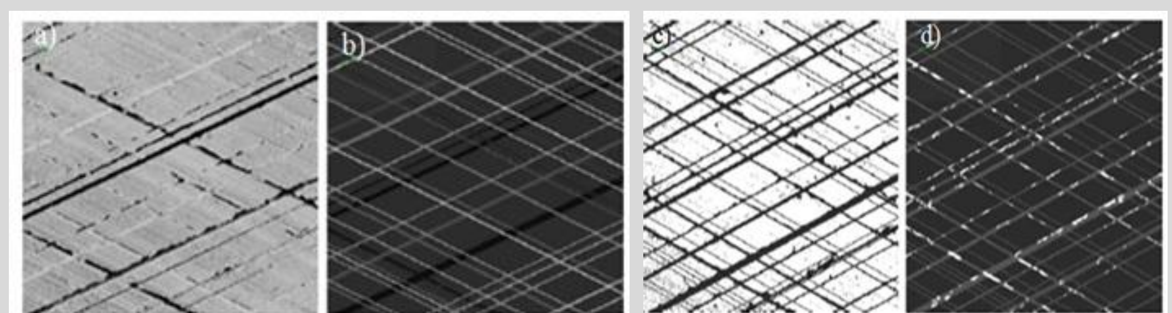
Fig. 3. Honing structure according to MBN 37800-1. From left (a) to right (d): original topography after the F-operator application, raster image, contact surface (white), undesired surface structures on the sheet metal part (white).
